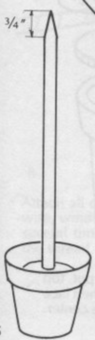
5 Sharpen the point of a wooden stick and paint it white. When dry, stand the stick in a flowerpot filled with sand or soil.
